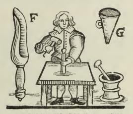
Fig. 2. THE MANNER OF DRIVING A ROCKET. (RICH CABINET, 1677.)
